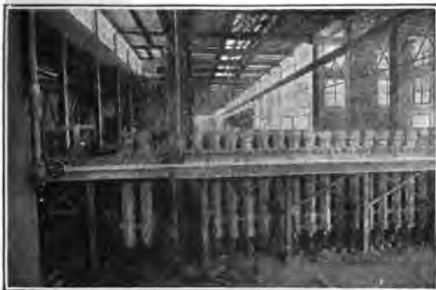
FIG. 190.—Drying Molds. Before the core can be placed, the mold must be thoroughly dried. This is done by either gas or coke fires.
